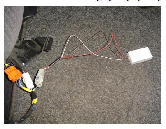
(5) Switch the ignition back on. The SRS light comes on and after a few seconds, it goes out. If the warning light comes back on after it had gone out, keep the ignition switched on for approximately 5 min. until the SRS control unit detects the emulator. Once the emulator is detected, the SRS light should come out.
