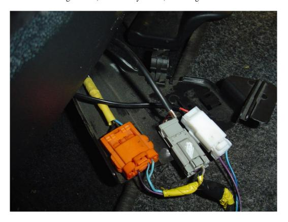
(3) Cut the OCS cable in a convenient place
