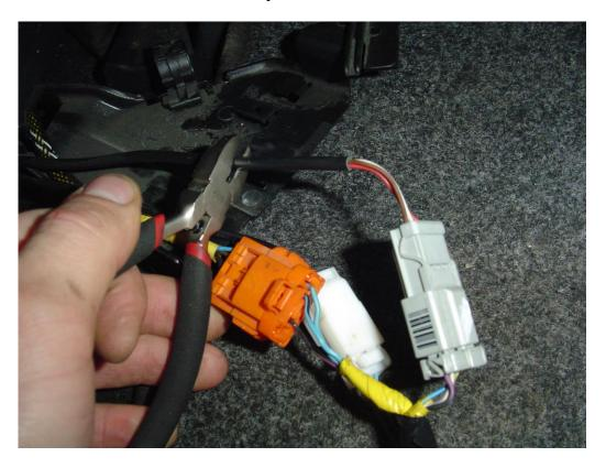
(4) Connect the emulator to the connector accordingly: signal to signal, ground to ground, positive to positive.
